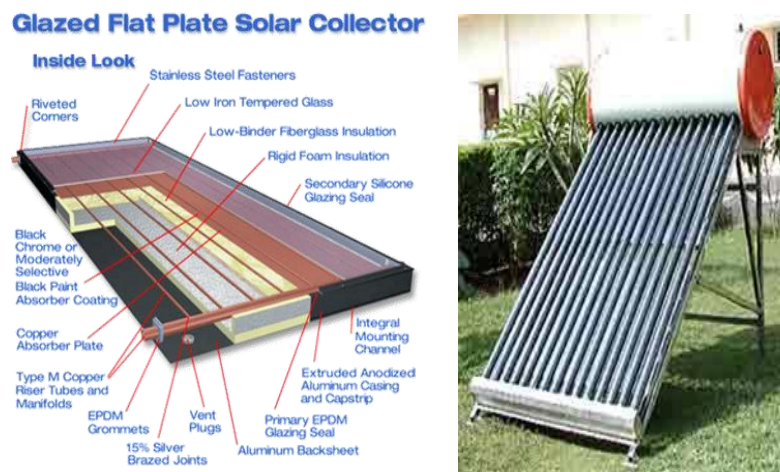
Fig.3 .Flat Plate liquid collector
